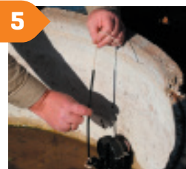
Apply anti-tangle tubing to the cord.
