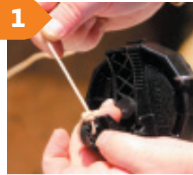
Secure one end of cord to the float arm.
