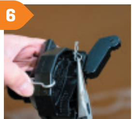
Replace the R-clip securing the lever, then follow steps 1-8 above.
