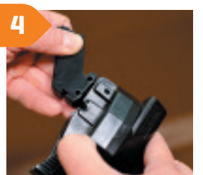
Invert the lever arm ensuring the lever points to the bottom of the valve.
