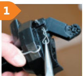
Using pliers remove R-clip that secures the pivot pin.
