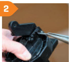
Using pliers remove the pivot pin.
